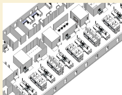
Top: Old chemistry labs with low exhaust capacity and irregular layouts. Bottom: Partial plan of renovated Chemistry Building that generates 20 percent more laboratory capacity.
